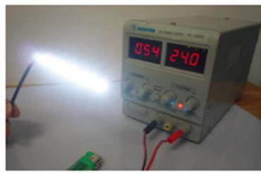
54mA Current before heating
