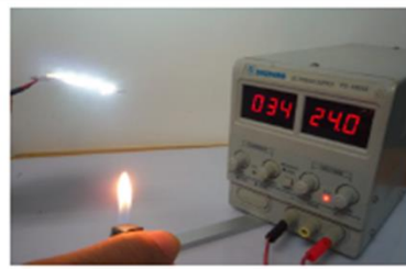
34mA Current when temperature get up
